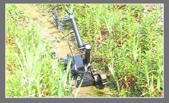
But resistance to rain and humidity are not the only reasons to need a waterproof UGV. You will need to clean your UGV and be confident that the cleaning process will not cause any damage. Zeus' ruggedised design allows cleaning with hot and cold low pressure water, steam, and detergents, without wear, deterioration, or damage.
