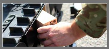
warning is sent to the operator to bring the UGV back to a safe point. Once the warning is activated, Zeus can still travel at least 500m ensuring it can be brought back to a safe place to change the battery before communication is lost. The OCU has the same low battery warning system enabling the OCU battery to be changed at a convenient point during the mission rather than at a critical point.
