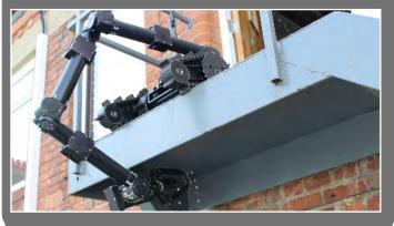
In addition, the gripper or claw can hold small tools and allows for the separation of the components of a suspect device after disruption. Examination with the through gripper camera permits confirmation the disruption has been successful.
