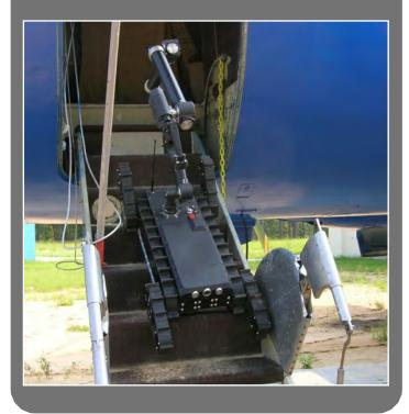
Track throwing, especially in hot weather, when traditional rubber tracks can stretch, is eliminated due to the Aramid reinforced rubber. This makes it almost impossible for the track to expand and jump off the driving sprockets.
