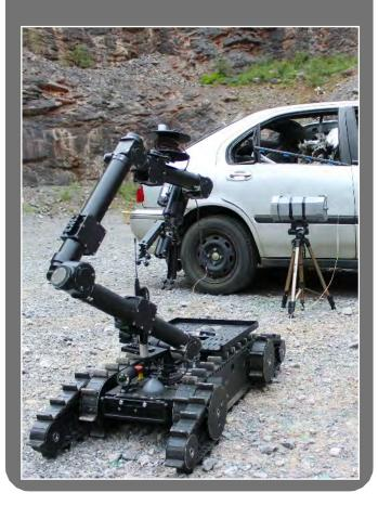
BootBanger, a very heavy tool, also presents no problems for Zeus. Delivered on the UGV chassis, held in a simple bracket, once on target, Zeus' strong arm lifts and positions BootBanger into place.
