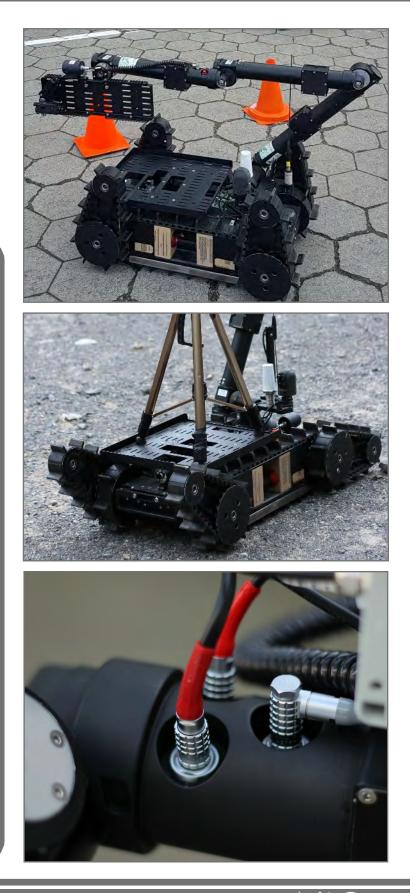
If you need to communicate with your additional tools, such as CBRNe sensors, data ports also are located on the chassis that can communicate with a wide range of protocols without the need to fit additional radios or tethers. Not only can you control your equipment, but data may be passed out and back to the OCU using the UGV's communication system. Once the data is back at the OCU it may be logged or
