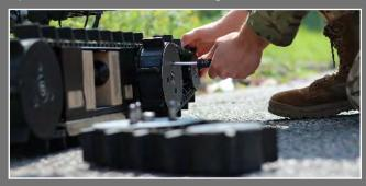
You also do not want to spend excessive time on preventive maintenance, and Zeus supports you here as well. User preventive maintenance is literally reduced to simply keeping the UGV clean, checking tracks, maintaining batteries and checking all functions are operating correctly.
