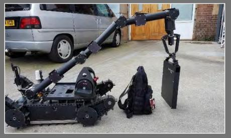
Zeus has a universal X ray holder system that can hold a wide range of X ray generators and plates from many different manufacturers. X Ray generators may be either held in the universal frame or chassis mounted for optimum performance.
