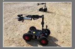
This modular design also allows you to replace your entire communication system if it became damaged. In a matter of minutes this subsystem can be swapped out by the operator and does not require a trained technician. This keeps Zeus up and running and on task.
