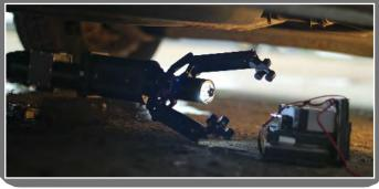
When aiming barrelled disruptors you will need to be able to judge distances accurately for maximum disruptive affect, and Zeus' laser aiming system viewed through the cameras will allow this. Even aiming stand-off disruptors up to 30m away using cameras and no lasers is possible with Zeus' unique and patented capability camera stand-off aiming system
