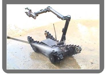
Water entering sockets or connectors is not a problem as they are all waterproof when mated or fitted with a blanking cap.
