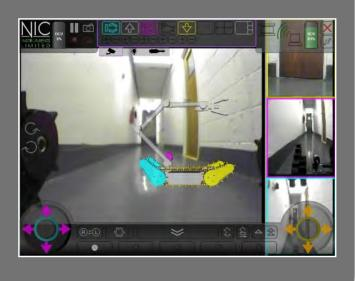
All ambient light conditions can be accommodated by the camera lights, including Infra-Red which are controlled from the OCU.
