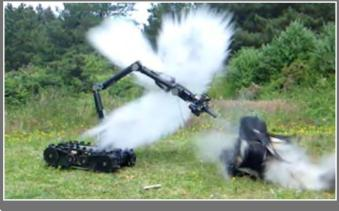
You need to position and aim disruptors quickly and accurately. Zeus' long and dexterous arm can reach up to 2m in height to fire disruptors horizontally for example into airplane overhead lockers. Viewing the potential target and the barrel of the disruptor is possible with the 5th camera that can be mounted onto the universal disruptor holder. The disruptor can also be viewed through Zeus' other cameras, including for example the pan tilt, to maximise your situational awareness.
