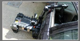
This dexterity allows the arm to reach below Zeus as well, so searching culverts, under bridges, ditches, or even digging into soft ground is easy. Tasks such as opening vehicle or building doors, boots of vehicles and gripping small objects requires precise control, and Zeus delivers this.
