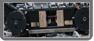
You need powerful lightweight batteries, and lithium lon currently offers the best power to weight ratio & availability. The charger supplied with Zeus can charge 2 batteries at once, and can also carry out battery conditioning, crucial to good battery management. Local voltages present no problems as the charger can work at 220V/110V and 24V/12V.
