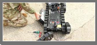
You may bring in a new or upgraded capability and need to be sure that your UGV is future proofed to be able to accept these new systems. Zeus' modular design has growth potential for future improvements, for example integration of new techniques or devices; upgrades or integration of new software without a negative impact on safety, performance, functionality or lifetime.
