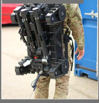
It also allows the unit to be stored more easily within vehicles, utilising multiple small cavities if space is at a premium, instead of one large one. It means that often a dedicated slot for the UGV is not required, and it can be placed under benches or alongside other equipment, meaning you can carry more capability in your vehicles.
