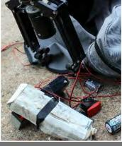
The ability to position a disruptor correctly to enable maximum disruptive effect (for example corner to corner on a bag) and within 2cm of a suspect device, is easily achieved.
