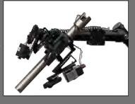
Zeus' unique disruptor mounting system allows you to maintain the claw on the end of the arm. This maintains and maximises your capability.
