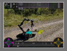
Many UGVs lose the gripper functionality when a disruptor is placed at the end of the arm, but Zeus' unique method of disruptor mounting means you can maintain full use of your gripper during a mission while a disruptor is mounted.
