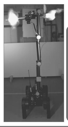
Stand-off firing is recognised as one of the hardest tasks to achieve when firing a disruptor from a UGV. Many systems try to use high powered lasers, but not only can these be hard to see on most terrains (especially outdoors) but can present safety risk to the operator.
