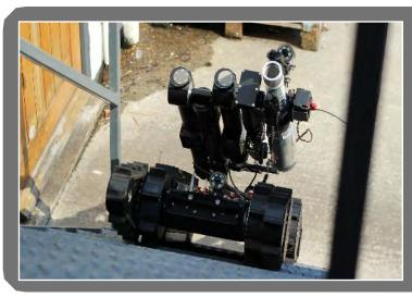
Zeus' unique track design allows it to 'lift' the entire UGV up stairs and obstacles as opposed to traditional UGV tracks method of relying on 'hooking' onto obstacles. This whole new concept in climbing gives unparalleled stability and control whilst climbing. Ditches, trenches and holes also present no problems as the articulating track modules easy broach such features in the terrain.
