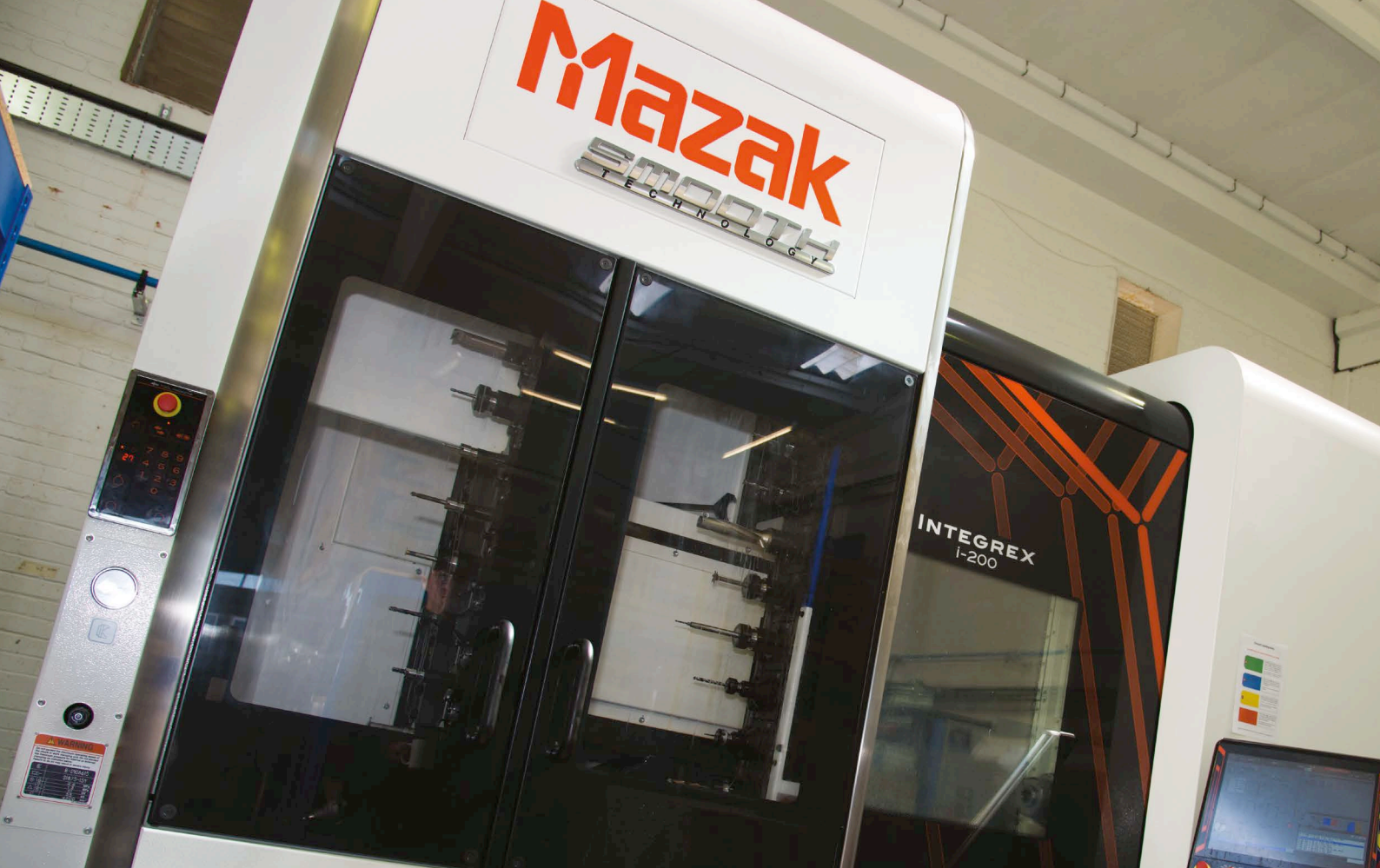
5-axis Mazak Smooth mill / turning machining centre
