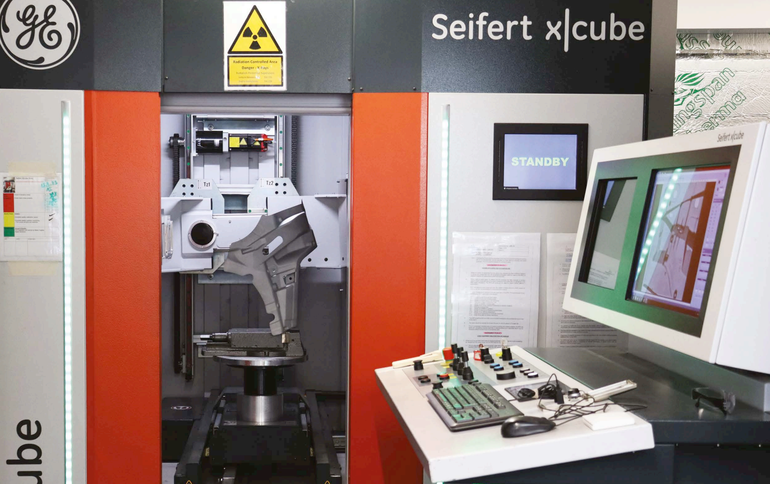
GE Seifert X|Cube 320KV scanning system
