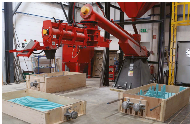
15 tonne per hour sand mixer
