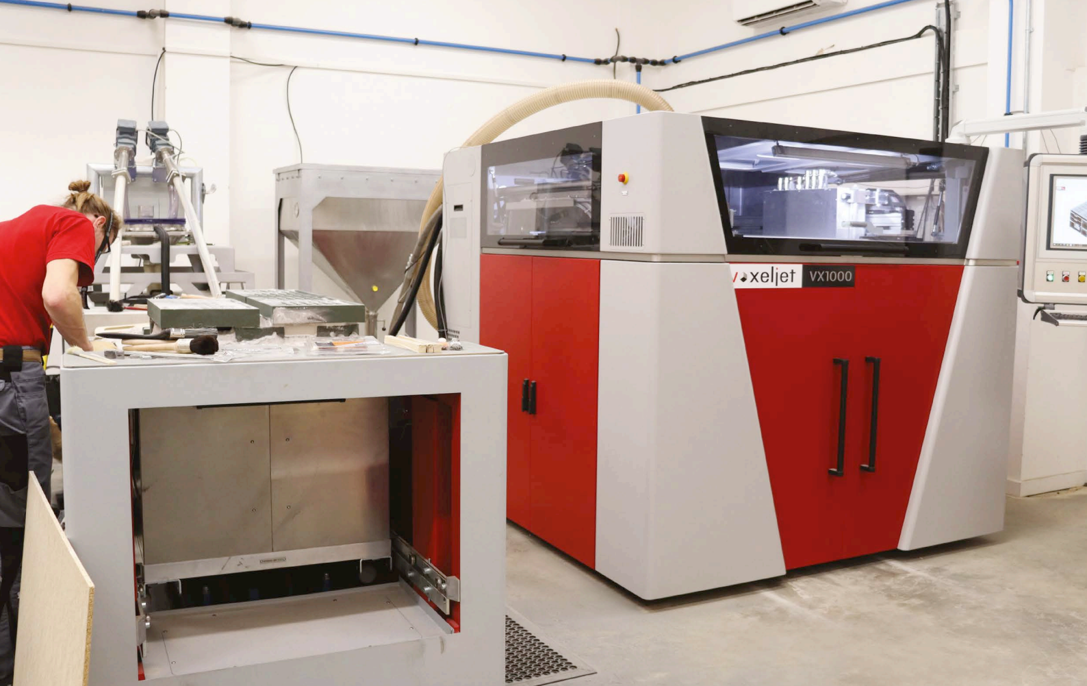
3D sand printing facility in operation
