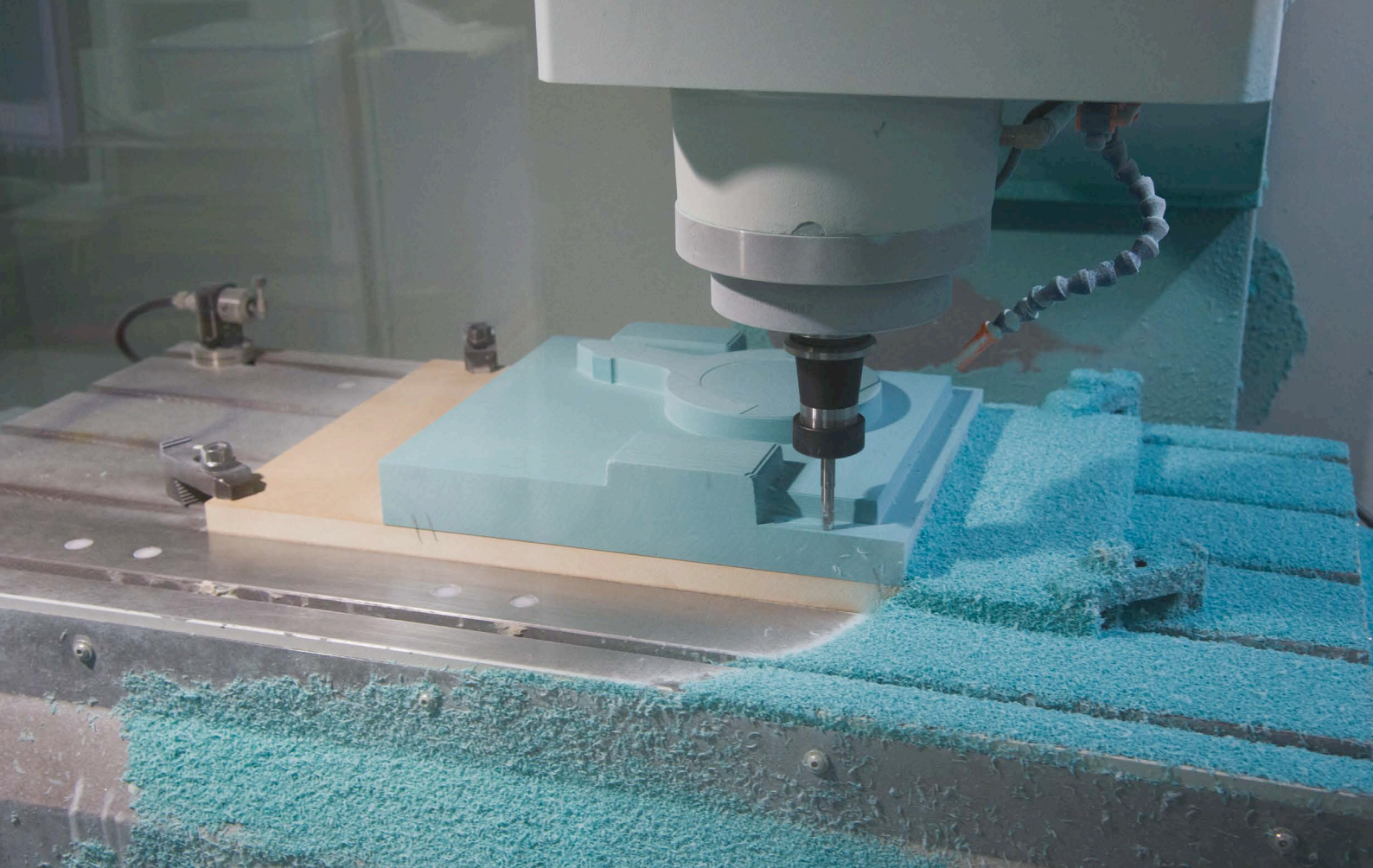
Machine cut pattern tooling
