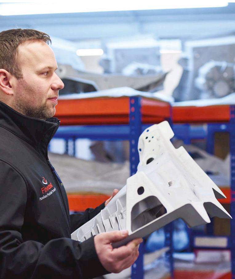
Completion of 2.5 mm wall shock tower castings
