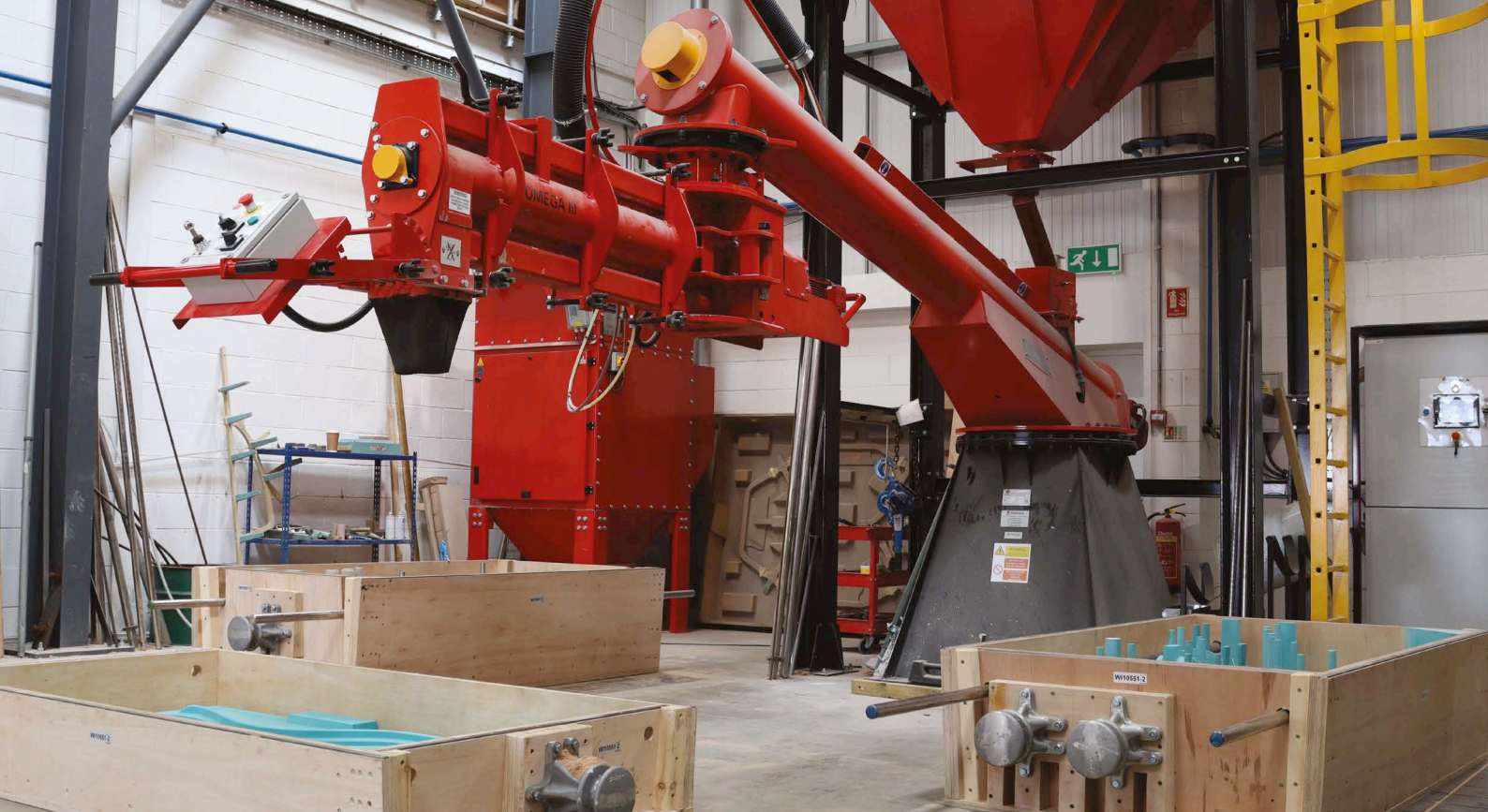
Two arm 15 tonne per hour sand mixer for extended reach and coverage
