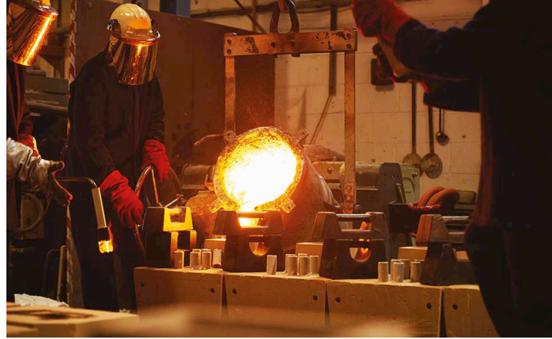
Pouring austenitic stainless steel castings
