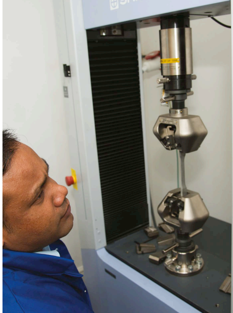
Tensile testing of sample test bar
