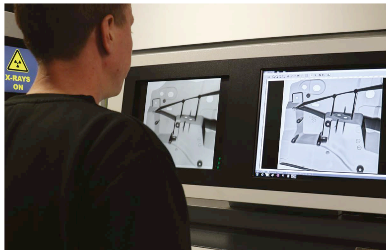
Digital radiograph review of cast component
