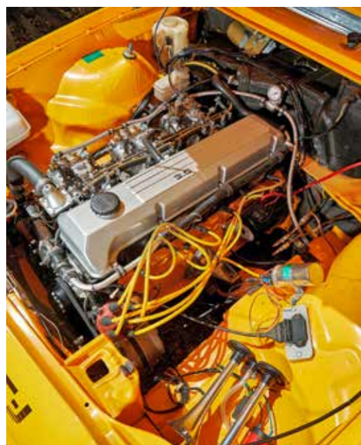
LEFT Clive made the manifolds by adapting original parts from the old Monza manifold.
