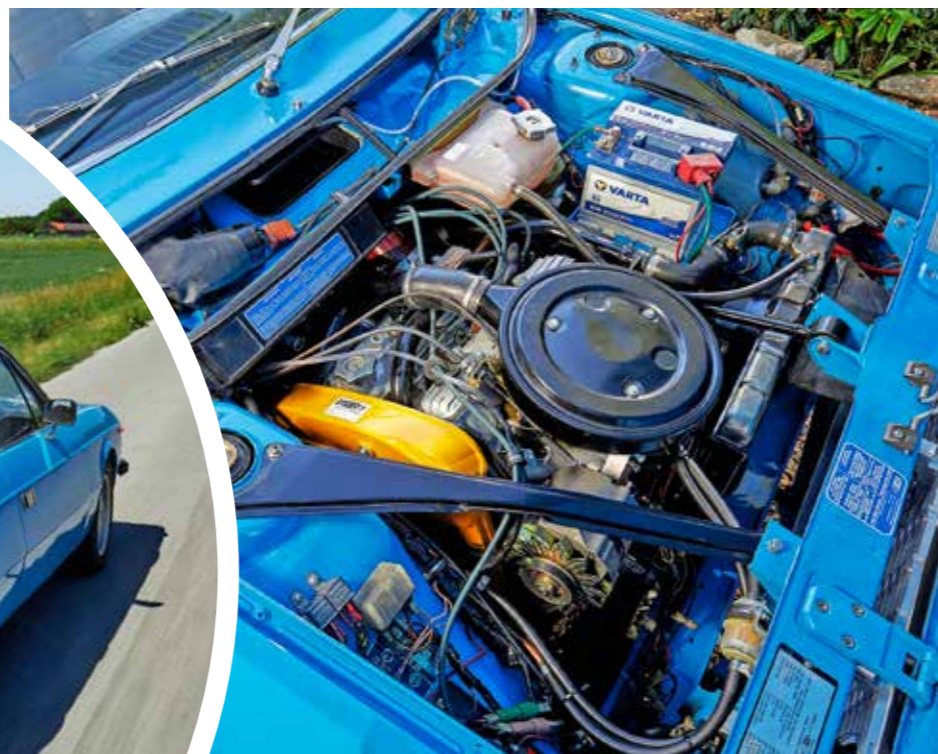
BELOW RIGHT Better-than-new 1995cc V4.
