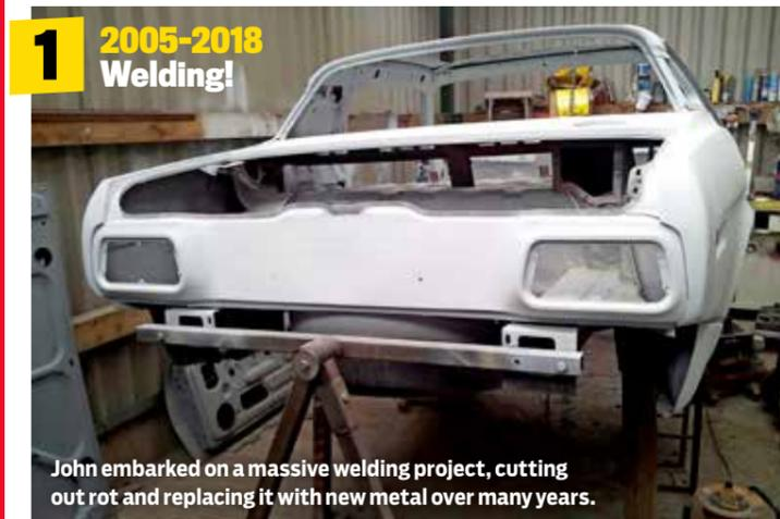
John embarked on a massive welding project, cutting out rot and replacing it with new metal over many years.
