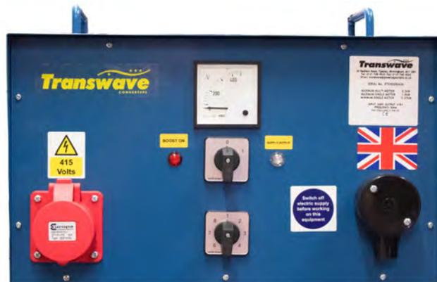
Care should be taken with the connection of the machine to the output plug/socket. If the machine has a contactor starter the 400/415v control coil must be fed from the phases marked L1, and L3. If the control circuit is fed incorrectly (i.e. connected to the phase marked L2) the contactor will either not operate or chatter when operating. Similarly, a control transformer and/or lighting transformer with a primary winding of 415v must be fed from the L1 and L3 phases.
