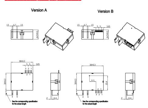
Note: 1.For single coil, the pin marked as dotted line; 2.No dimensional tolerance noted:±0.3mm.
