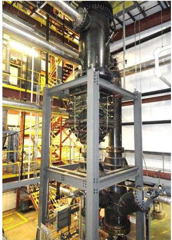
250 kW t fuel direct chemical looping test unit
