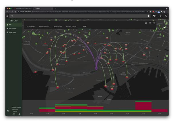
Utilihive SMOC combines data from the Head End System(s) (HES); network device, communication performance information, fault information from the telco provider, network topology information from the GIS and other reference data from the System-of-Records (SOR) to provide a holistic view of the AMI and communication network status.
