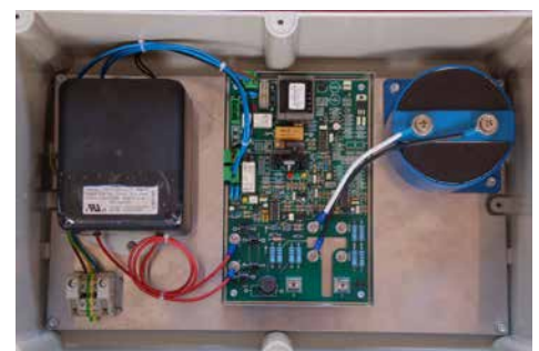
Heavy Duty power unit in Safe Area enclosure
