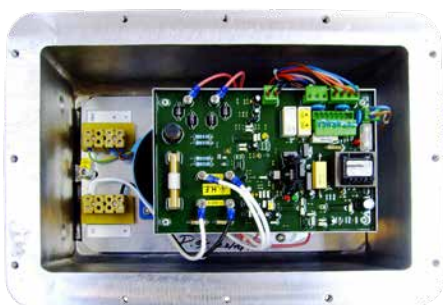
Heavy Duty power unit in certified ATEX enclosure
