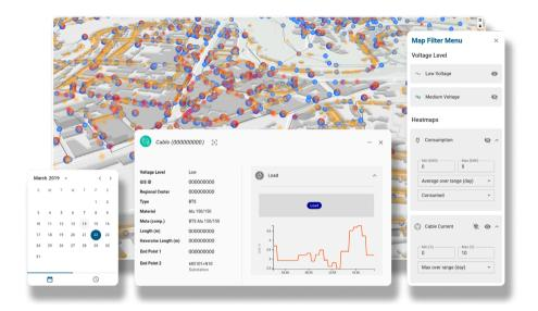
Not only does it integrate **power-flow calculations**, but it also rationalizes maintenance scheduling and mid-term transition-related investments. It allows **simulation** and **planning** of the effects of any potential grid adjustment, such as new infrastructure commissioning or (un)scheduled reparations.
