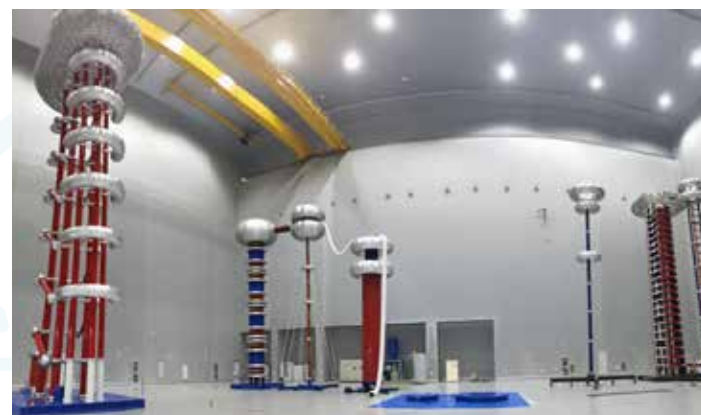
1000kV AC breaking testing lab and \pm 800 kV DC breaking testing lab
