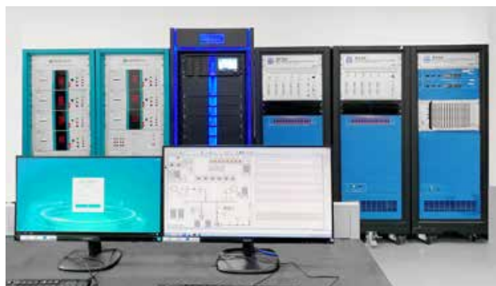
The RTDS simulation system for ultra-high voltage protection and power electronics
