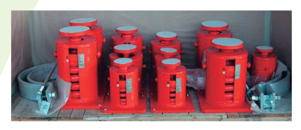
Ca.S.T.Im. 2000 supports with a variable load are manufactured in three series of total working strokes (45 - 90-180 mm). Each series has seven different execution types which satisfy different installation requirements. For each type, we manufacture 22 different sizes having rising capacities between 19 and ~22000 daN.
