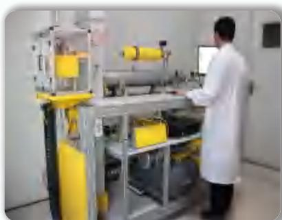
AFC-133 Filter Material Dynamic Test Platform (Germany)
