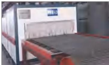
Mesh-belt Type Sintering Kiln
