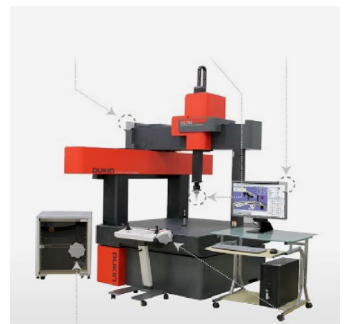
3D measuring machine (measurement and verification of processed parts)
