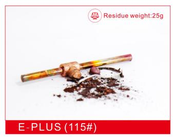
Only joints, a small amount of welding slag
