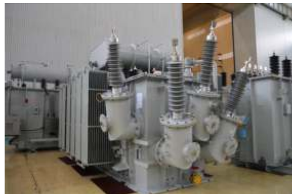
State Grid Shandong Electric Power Equipment Co., LTD Mengdong 66KV Mobile transformer SZ11-2000/66
