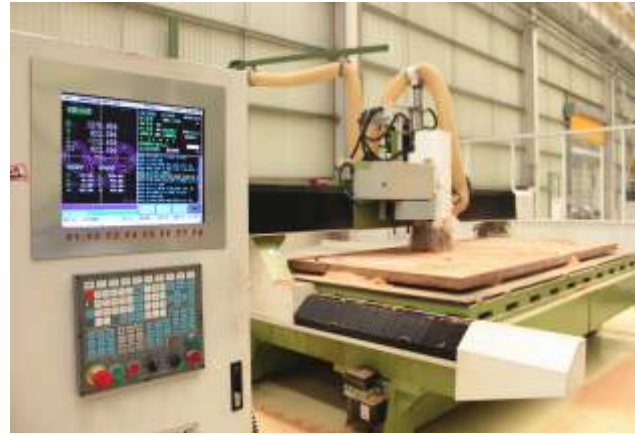
CNC insulation processing center
