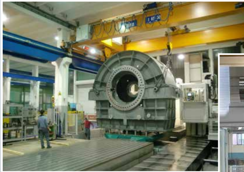
STEAM TURBINE CASING
