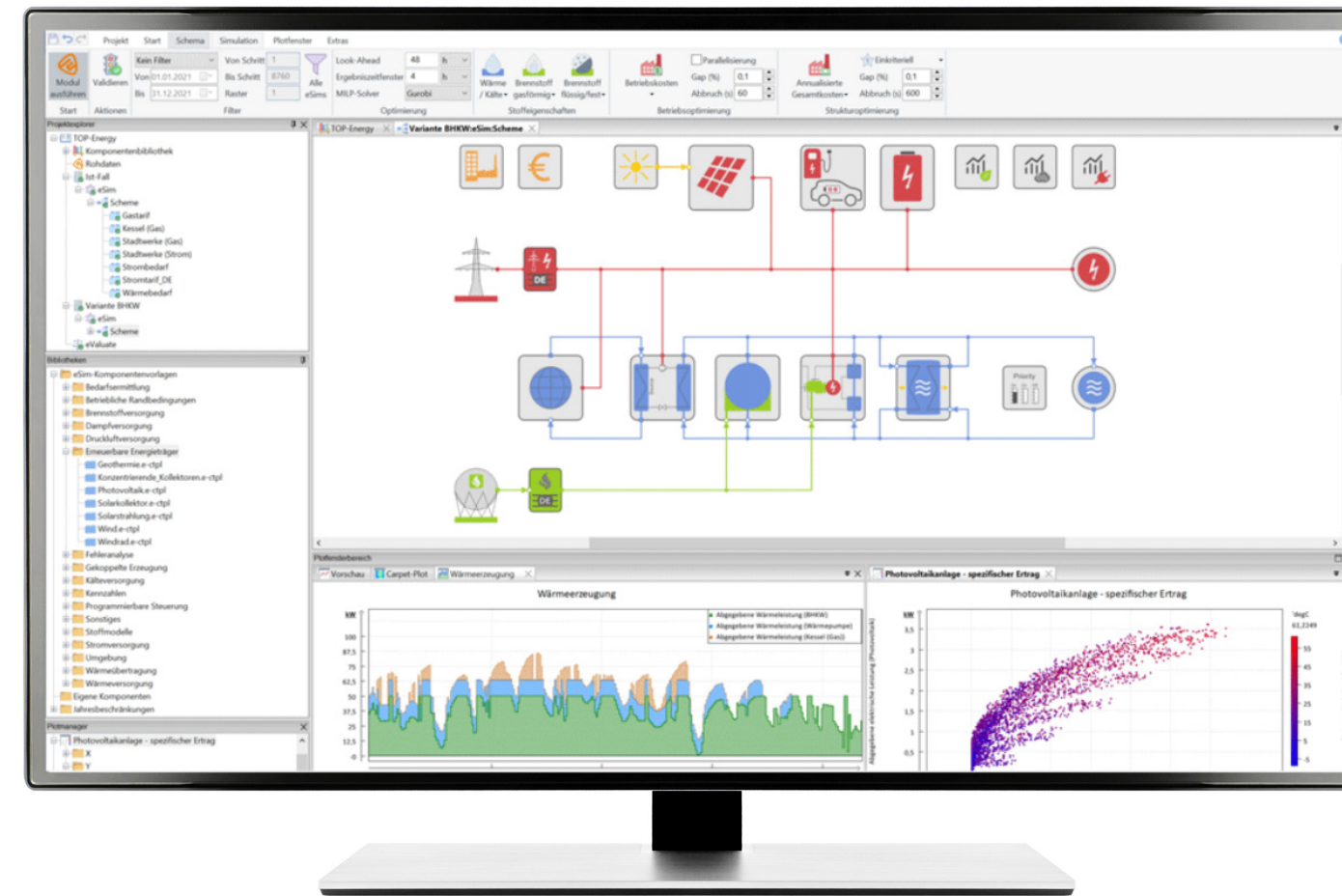
Potential analysis - integration of an energy storage device and PV into the building energy system
