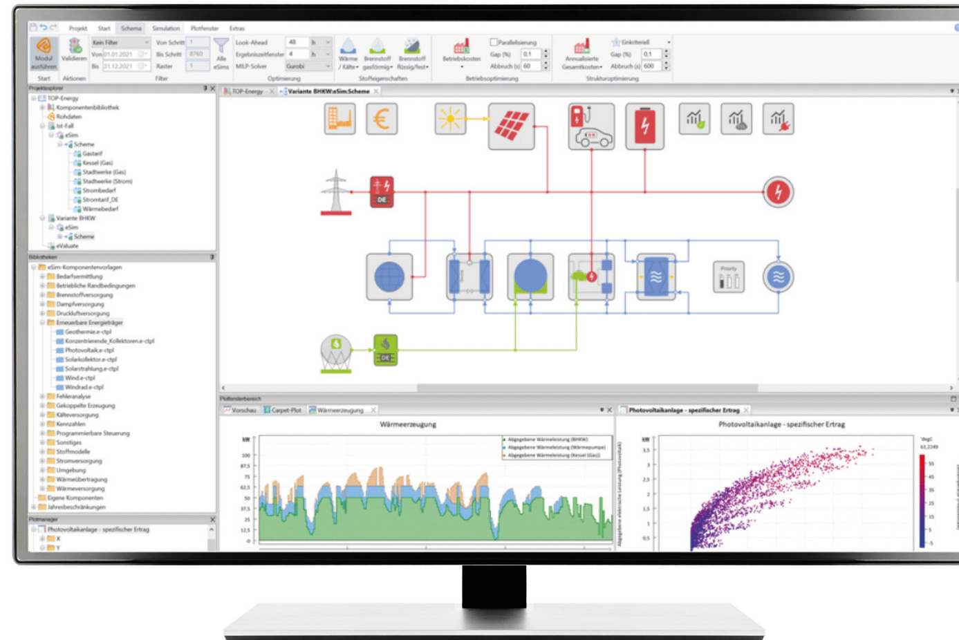
Potential analysis - integration of an energy storage device and PV into a buildings energy system
