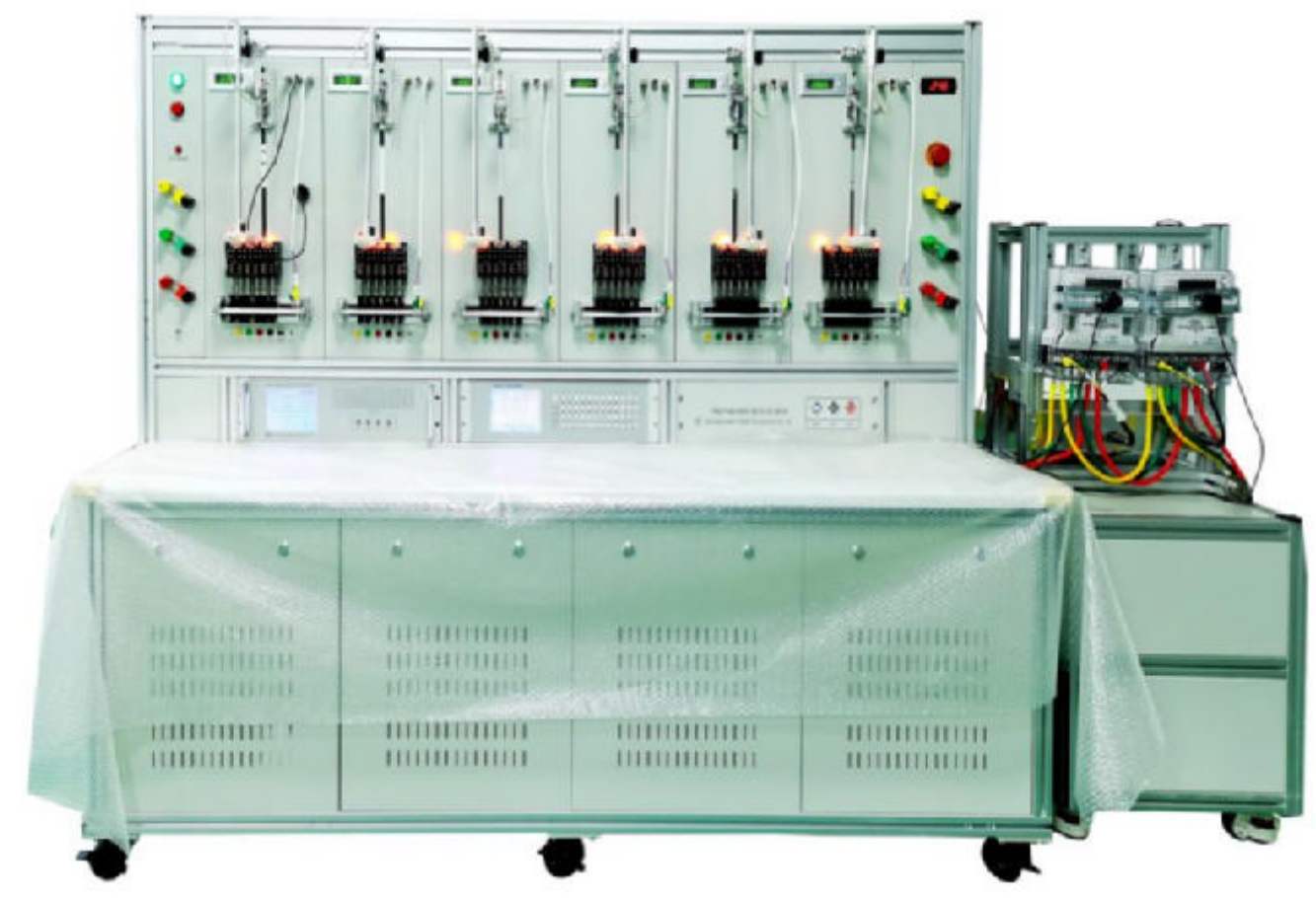
3PH Meter Test Bench for R&D lab
