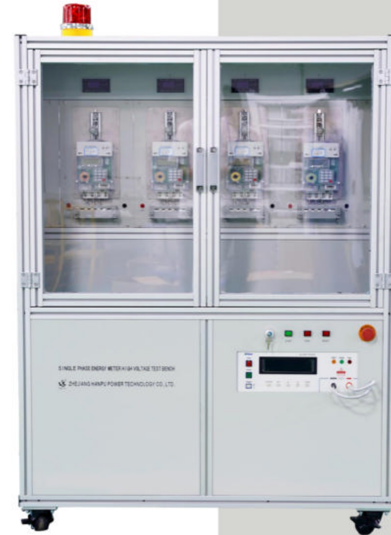
1PH/3PH High Voltage Meter Test Bench
