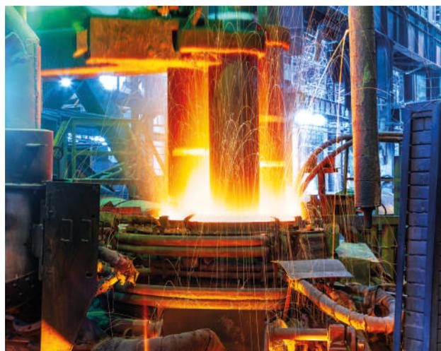
*Replacing blast furnaces with electric arc furnaces is a major stake for decarbonizing steel production.*
