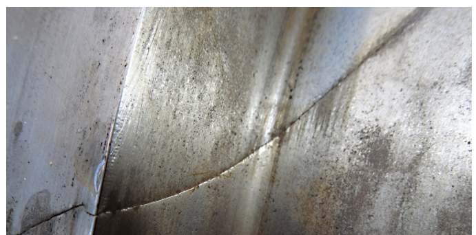
Excessive amplitudes of torsional vibrations can lead to shaft cracking without warning.
