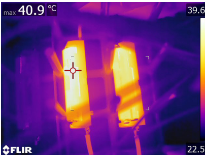
Heating up of a battery cell during a rapid discharge, measured by infrared thermography
