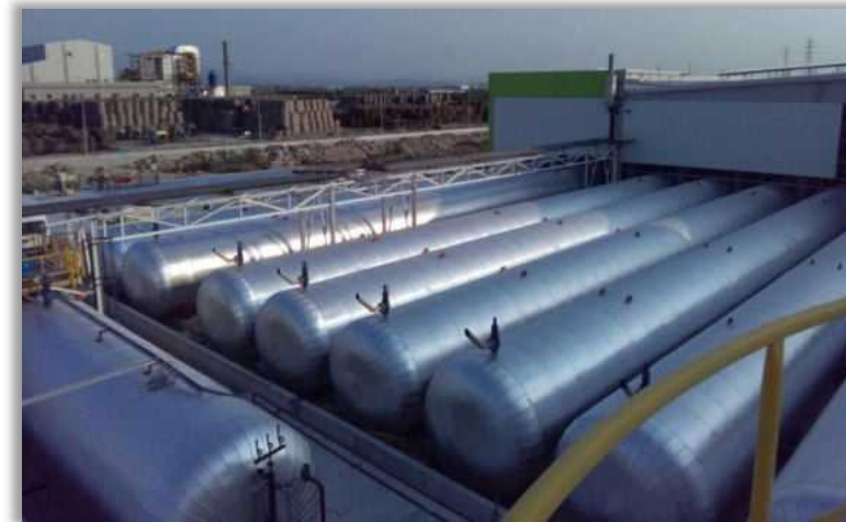
Ø 2.900mm x 16 bar x 45 mt Autoclaves
