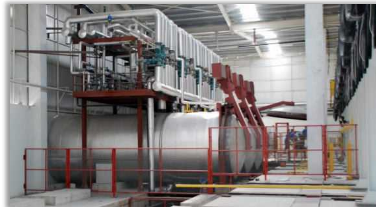
Ø 2.900mm x 16 bar x 45 mt Autoclaves
