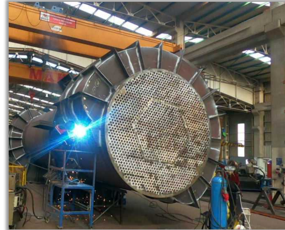
120 ton weight Sulpuric Acid Process Heat Exchanger
