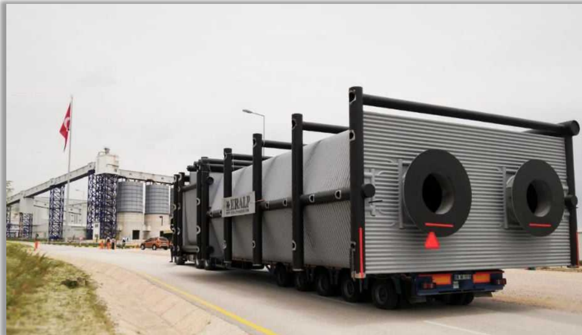
90 ton/h 55 bar 450°C Superheated Water Tube Steam Boiler
