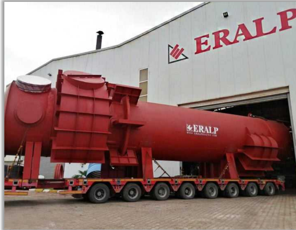
120 ton weight Sulpuric Acid Process Heat Exchanger
