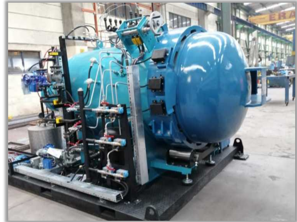
20 Bar Operating Pressure, 400°C Composite Autoclave
