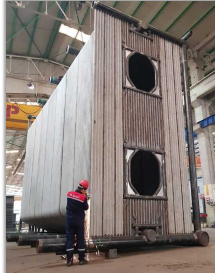
90 ton/h 55 bar 450°C Superheated Water Tube Steam Boiler
