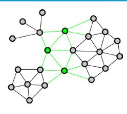
Communication via multiple nodes - better network throughput, in case a green node fails, there is an alternative path.
