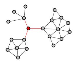
Communication in the network takes place through a bottleneck - low throughput, the failure of a red node will cause the loss of a large part of the network.
