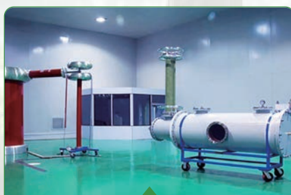
05 Fully shielded 350kv partial discharge-free power frequency test laboratory.
