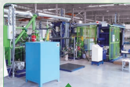
03 Germany imported HEDRICH epoxy resin automatic pressure gel production line.
