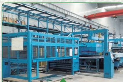
02 Japan imported Murata sheet metal flexible processing production line.
