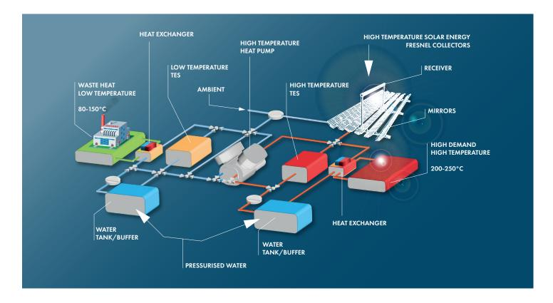
SUSHEAT uses waste energy available in the industry to charge low-temperature thermal energy storage tanks, which are upgraded by the HT-HP and stored at high temperatures. The HT-HP can also upgrade ambient heat and solar energy, initially to low temperatures, and later to high temperatures.
