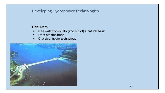
Tidal energy can be harvested through tidal dams and turbines to capture the energy as head energy.
