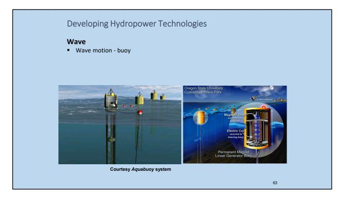
Energy in waves can be harvested, for example with these wave elevation capture devices.
