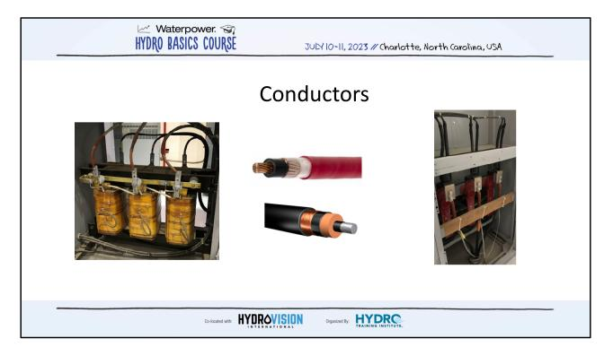
Main Point: Conductors are made of a variety of materials based on the intended application. A good conductor allows electrons to freely move through the material. Hence copper makes a quality conductor because it has 1 electron in the outer valence shell, therefore its waiting for a force like volage to induce them to move. On the opposite side of the spectrum, Rubber acts a quality insulator because it does not allow electrons to freely exchange.
