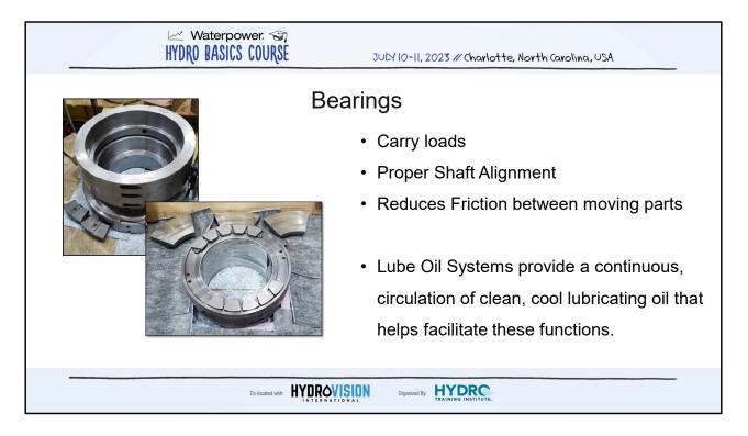
Main Point: Bearings assist rotating equipment and are designed to carry loads, provides proper shaft alignment and reduces friction between moving parts. Proper bearing lubrication is extremely Important.
