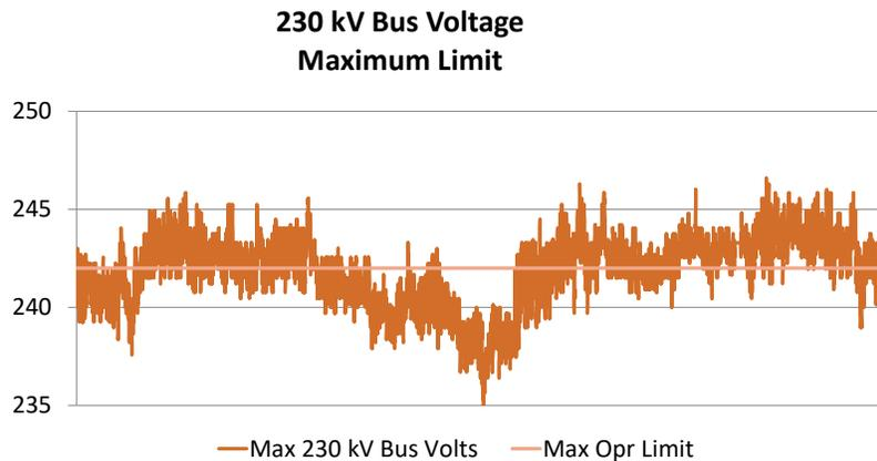
The last item is the voltage support required at times in the system. This plant is located on a long, lightly loaded line during parts of the year due to water for hydro units. Forces units to operate at relatively high power factors and stability limits. More risk to machines by operating at fringes of design limits.
