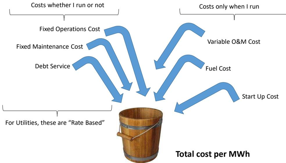
Generator Dispatching – this is an economic decision in most cases. To determine the economics, there are several factors that contribute to the cost. This cost is divided by the MWh's produced and is used to determine the cost for generation. The lower the cost per MWh, the more economic the choice.
