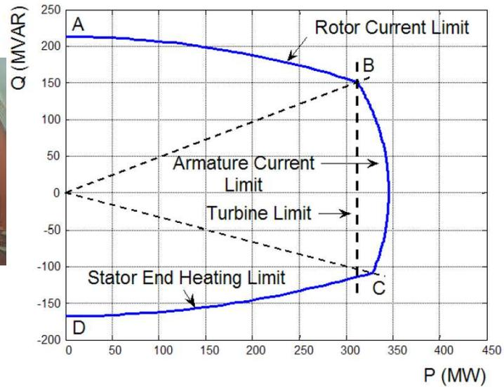
Real and Reactive Power capability. This shows how much a reactive energy can be provided by a generator. What is important is that the reactive power (Q) is dynamic and is capable of adjusting automatically depending on what the system demands.
