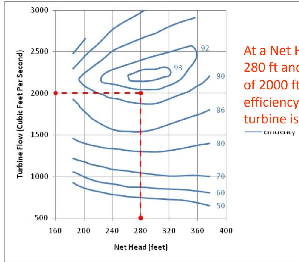
At a Net Head of 280 ft and a Flow of 2000 ft<sup>3</sup>/s, the efficiency of the turbine is 91.5%.
