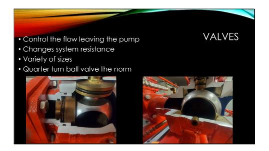
Quarter tune ball valves are the most common valves used on fire apparatus, they are compact, few moving parts, and relatively inexpensive. The main components are the ball and seat. If the seat is damaged water will leak by when the pump is engaged. This is why it is important to open the drains on a regular basis. Water coming out from the drain is an indication the valves are leaking. When a valve is leaking it will not pass the annual pump test, vacuum test with caps off.
