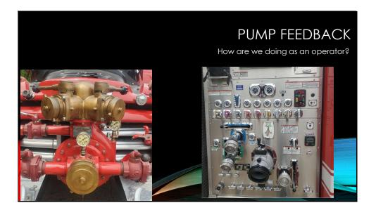
The pump panel has definitely evolved over the years, from a single input and output gauge to multiple gauges and displays provided a wealth of information to the operator.
