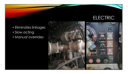
Electric valves are used when the location will not allow linkage to be ran, or the valve needs to be slow acting.
