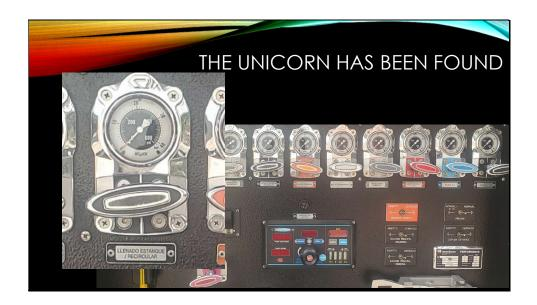
Company 18 in Santiago Chile has a tank to pump pressure gauge. This is the only one I have seen.
