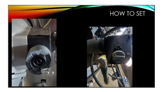
Some styles of relief valve have a stepped ring on the outside of the stem marked with pressure values, when the stem is aligned with the step the valve is set for approximately that pressure. The other style of relief valve is an adjustable stem and lock nut. This style requires a pressure gauge to know the opening pressure of the valve when setting.
