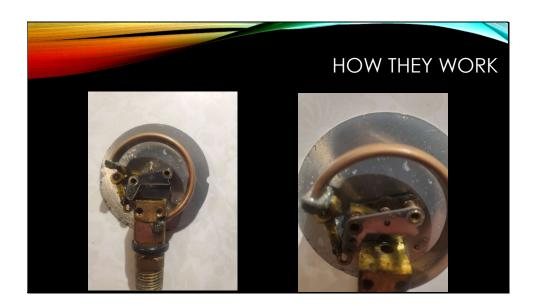
The Bourbon tube pressure gauge was invented by the French Scientist Eugene Bourbon in 1849. It consist of a C shaped tube, linkages, gears, and pointer. The tube when pressure enters, the amount of deflection is based on the material and construction of the tube. The deflection of the tube then pulls the linkage which turns the gears connected to the pointer. Once the tube is damaged, from freezing for example, the gauge will not return to its original condition.
