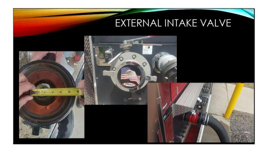
External intake valves have waterways smaller than the 6 inches intake piping. The main styles of intake valves are piston, butterfly and ball intake valves (BIV). Piston valves, and ball intake valves are external to the pump intake plumbing. Butterfly valves can be external or integrated into the intake plumbing.
