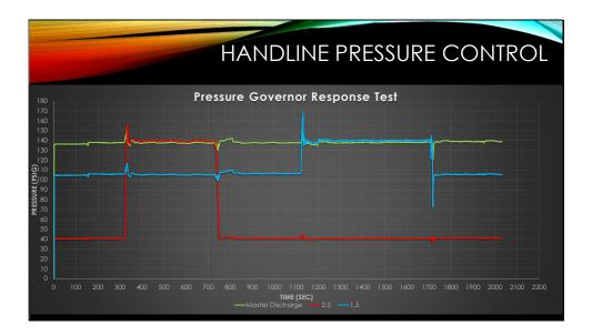
This chart shows the response of the FRC pressure governor in PSI mode to opening and closing different size lines.
