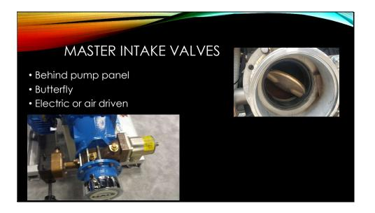
Master intake valves are butterfly style valves the same size as the intake waterway. The valve is operated by electric motors or air actuators.
