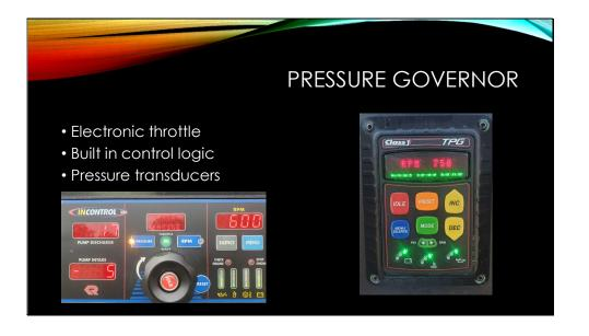
Pressure governors use the chassis fly-by-wire throttle and engine management system along with master discharge pressure transducers, and in some cases inlet pressure, coupled with control logic to manage the pressure generated by the pump.
