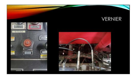
A second cable ran from the engine's throttle to the pump panel. The cable would increase the RPMs when it was shortened, turned counterclockwise, and RPMs decrease when it was lengthened, turned clockwise.
