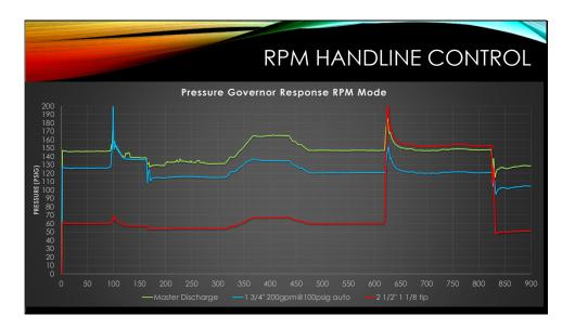
This chart shows the response of the FRC pressure governor in RPM mode to opening and closing different size lines.
