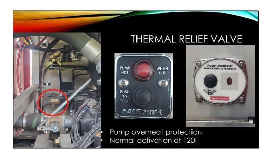
Thermal relief values use a temperature reactive spring which opens at 120F. Hard water can cause the springs to stick open once activated. The location of the thermal relief value is distant from the center of the pump meaning heat damage can occur to seals and bearings before the value may open.
