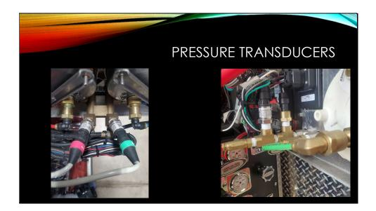
Transducers provide an electrical signal, usually 4-20mA, proportional to a calibrated pressure range. This is done by strain gauge on a diaphragm.
