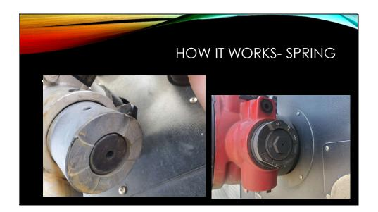
Most intake relief values operate with a spring holding a value to a seat. When the force on the value is greater than the force of the spring the value will open relieving the pressure. Turning the adjustment nut down increases the compression of the spring and the force exerted on the value requiring higher pressures for it to open.
