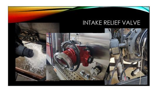
Intake pressure relief valves are located in two places along the intake, before each large intake valve and on the intake manifold.
