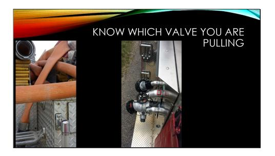
Opening the wrong discharge will slow the operation and potentially injury personnel. Verify the discharge being opened is the correct one. If needed, add additional labeling for easier visibility. Color of discharge label must match the color of the discharge handle. Color coding the hose to match will add another level of indication to the operator on the fire ground.
