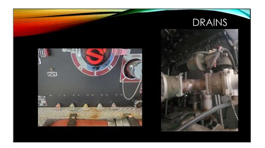
1900 13.8.1 A readily accessible drain valve(s) that is marked with labels as to its function shall be provided to allow for draining of the pump and all water carrying lines.
