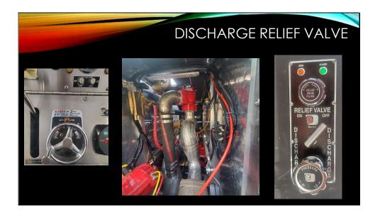
Discharge pressure relief valves dump excess pressure from the discharge manifold to the intake when the set point is exceeded. This protects the handlines from pressure surges when other lines are shutdown. The discharge relief valve vents to the intake line preventing water being seen on the ground when it opens unlike the intake relief valve. The lights are the primary indication if the valve is open or close.
