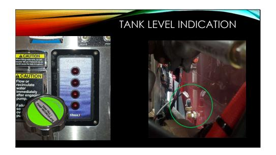
Most level gauges use a pressure transmitter at the base of the tank to determine the level by the pressure head.
