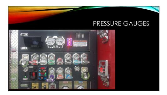
The pressure gauge is the primary feedback mechanism for the pump operator.
