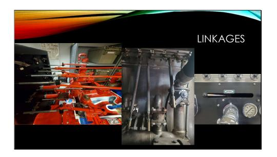
Linkages can bind, invert, or pins fall out. It is not a bad idea to have an extra linkage pin on the apparatus. If a linkage gets stuck, open the pump house to see if the linkage is inverted. If so, manually pop the linkage back inline. If it is stuck, remove the pin at the valve and try to move the valve directly.
