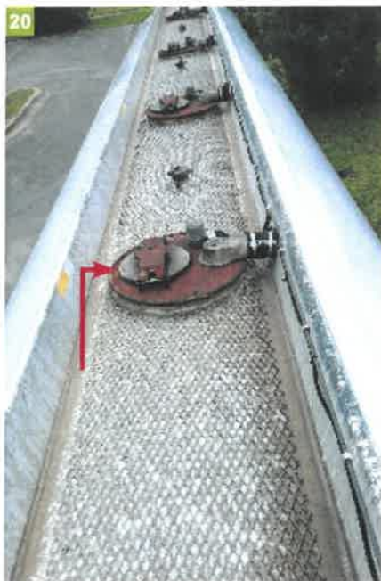
(20) On the manhole, clockwise from left (arrow) are the dome hatch, the Scully device, and the vapor valve.
