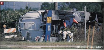
ness" of the tank end. This tanker was carrying hydraulic oil and was not properly placarded. The placard read "Drive safely." MC-307/407 tankers are usually an insulated, single-compartment, stainless-steel tank and have a thin aluminum "skin" on the outside.
