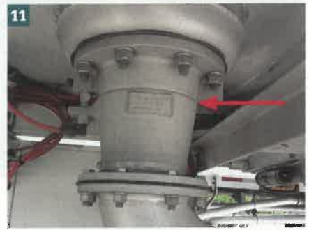
(11) Note the shear point of this air-operated belly valve housing (arrow). (Photo by author.)
