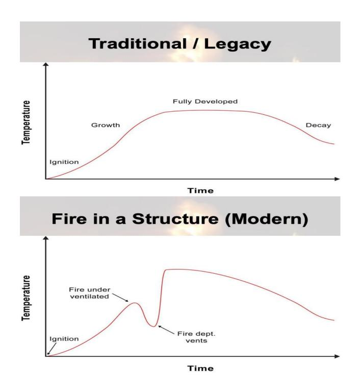
Due to more efficient sealed up structures, the fire is under ventilated and decays until the reintroduction of oxygen.
