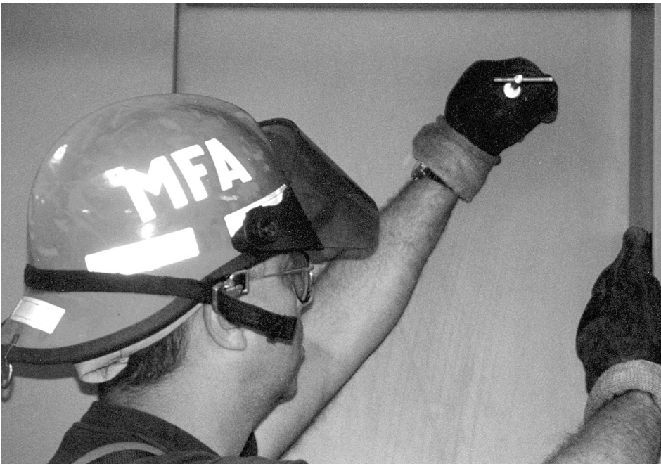
Fig. 1.3.4(b) Use of Hoistway Door-Unlocking Device
