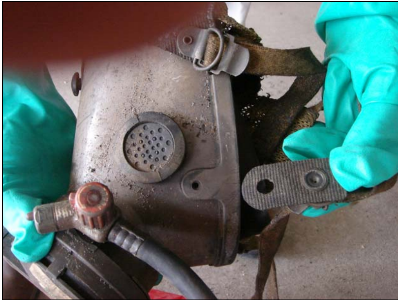
Photo 1. Facepiece missing a harness fastener. (NIOSH photo)
