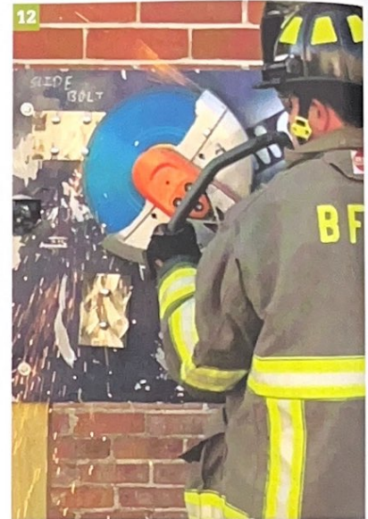
(11) Cut inward at a 45° angle to the bolt head, shearing in half the bolt inside the door. (Photos 11-12 by author.) (12) Notice the 1/4-inch steel plates mounted to the door surface. Shear off the heads at a near 90° angle. Notice the blade is set up in an outboard position, which allows the blade to get close to the door surface.
