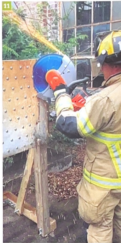
(11) Cut inward at a 45° angle to the bolt head, shearing in half the bolt inside the door. (Photos 11-12 by author.) (12) Notice the 1/4-inch steel plates mounted to the door surface. Shear off the heads at a near 90° angle. Notice the blade is set up in an outboard position, which allows the blade to get close to the door surface.
