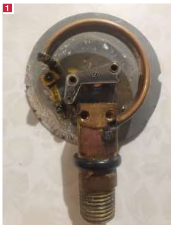
1 The inside of a bourdon tube pressure gauge. (Photos by author.)
