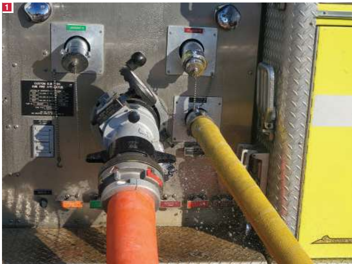
1 2 Examples of ball intake valves. (Photos by author.) 3 A ball intake valve waterway.
