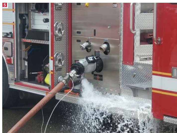
4 A master intake valve with manual override. 5 An intake relief valve under test.
