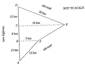
The old road from A to D (via F and E) is to be replaced with a new highway (ABCD). The diagram shows the new highway ABCD and the offset survey of the old road.
