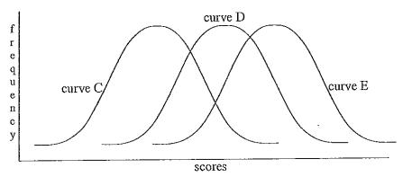
In the above diagram, the curves have the same standard deviation, but the mean, median and mode for curve D are more than those for curve C but less than those for curve E.
