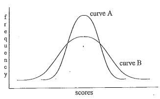
The diagram shows two distributions with the same mean, median and mode, but curve B has a larger standard deviation than curve A.
