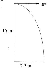
What would the initial velocity of the book have to be to hit the ground at that point? Use 9.8 ms<sup>-2</sup> as the acceleration due to gravity and neglect air resistance.
