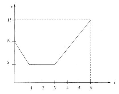
The graph above shows the velocity of a particle in cm/second. Find the total displacement of the particle in the first 6 seconds.
