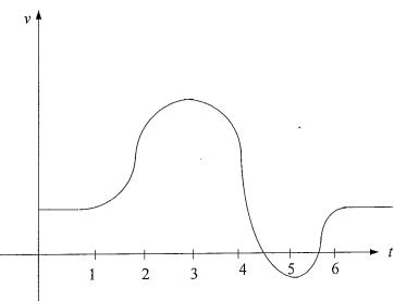
The velocity of a particle is shown above as it moves along a straight line.
