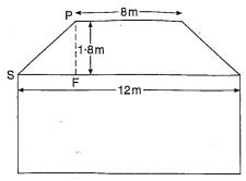
F is the foot of the perpendicular from P onto the base plane of the roof, and  $\angle PSF$  is the angle that PS makes with the horizontal.
