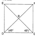
Since DEFG is a square, the angles in DBG will be 45°, with an angle of 90° at B. We know that DB = 0.8342...m, and that DB = BG.
