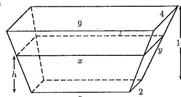
A solid has top and bottom faces which are parallel rectangles of dimensions  $9 \times 4$  units and  $3 \times 2$  units respectively. The altitude of the solid is 10 units.
