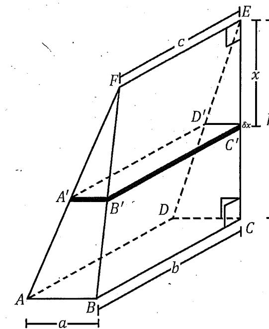
Consider a rectangular slice  $A'B'C'D'$  (parallel to the base  $ABCD$ ) which is  $x$  units from the top edge with width  $\delta x$
