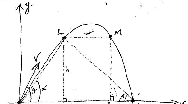
$$(a) \underline{\text{RTP}} \quad t_1 + t_2 = \frac{2V}{g} \sin\theta \quad \text{AND} \quad t_1 t_2 = \frac{2h}{g}$$
