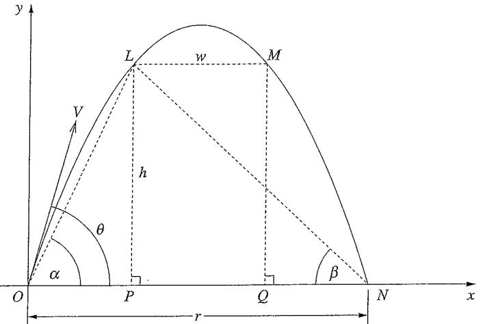
A projectile is fired from  $O$  with velocity  $V$  at an angle of inclination  $\theta$  across level ground. The projectile passes through the points  $L$  and  $M$ , which are both  $h$  metres above the ground, at times  $t_1$  and  $t_2$  respectively. The projectile returns to the ground at  $N$ .
