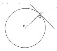
A Tangent meets a radius at its point of contact at right-angles.
